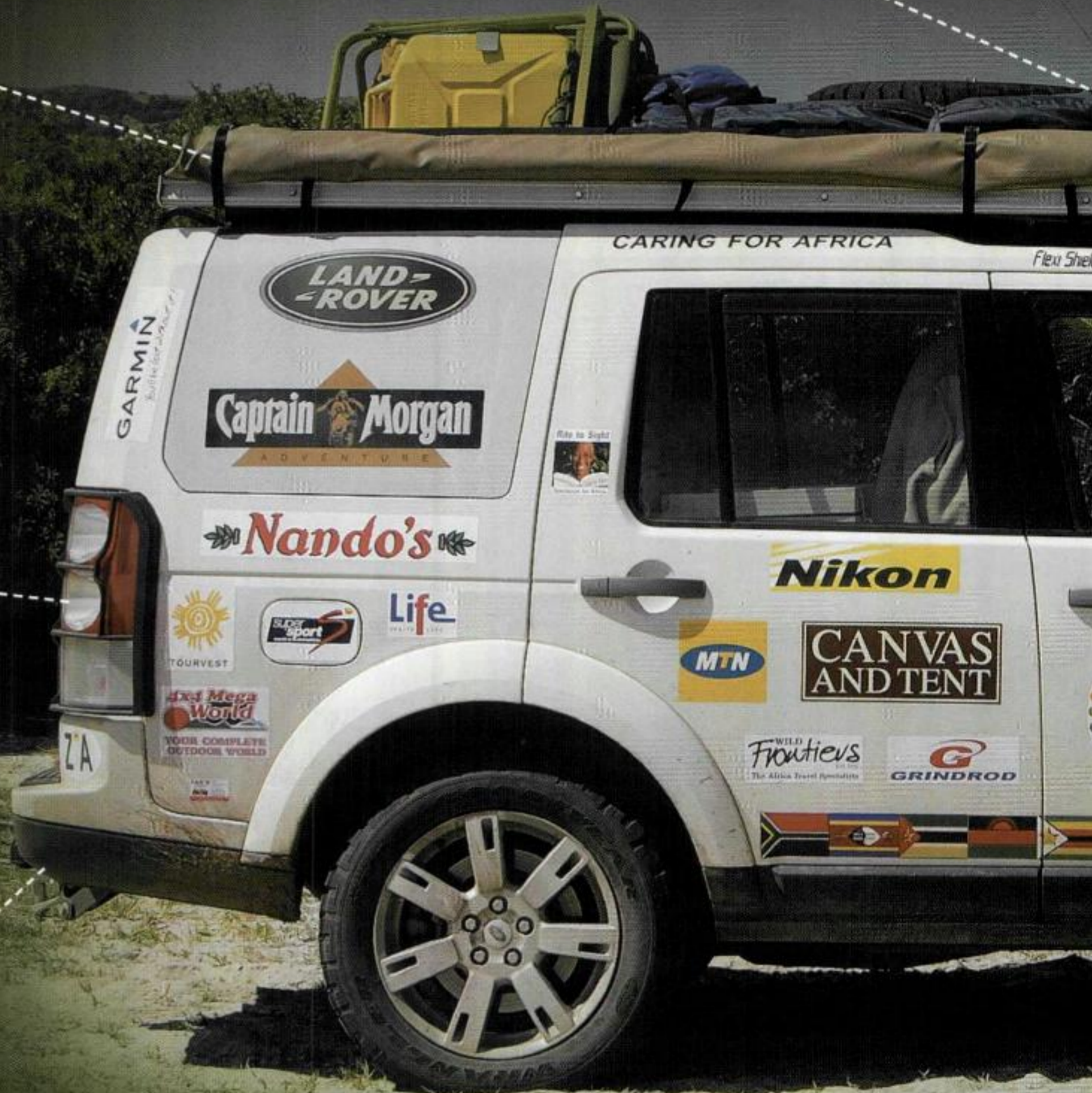
Expedition roof rack and ladder: The neat ladder provides access to the heavy-duty roof rack, which features additional reinforcement in order to cope with the abundant food, diesel, water and mosquito nets that are carried
