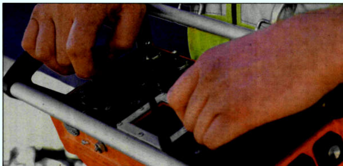
CONTROLLING THE SUPERSTRUCTURE. The 450-ton superstructure at the top of the tower of the GTK 1100 crane is directed from the ground via remote control. The first windmill in the planned wind farm at the Coega Industrial Development Zone was erected last week with the R70-million GTK1100 specialist windmill erection crane. Picture: Sabrina Dean.
